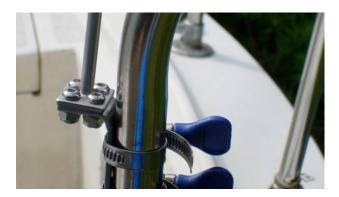
Use the L-bracket with the L upside down, which ensures that it can't slide out the bottom of the hose clamps. The L-bracket comes with special wing-nut hose clamps that can be tightened by hand without any tools.
